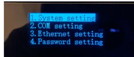
2. Next, use the Joystick to navigate (L-R-Up-Down) through the Menus, go to #2, COM setting.
