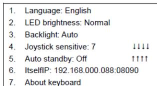
2. Move Joystick to #6 (ItselfIP), and then move to right to configure the IP of the CL01. You can use the CL01 number pad to enter digits.
